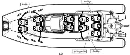
On the picture (Fig.D3.1) you can see the recommended location of the crew in the boat for **Design Categy C**. All persons should always use the handholds to avoid falling overboard. On Fig.D3.1 you can see the location of the handholds for each crew member. Any part of the boat can be a handholds that can be grabbed by hand to reduce the risk of falling overboard. Example handholds: handle, shroud, seat edge, cleats, steering wheel.
