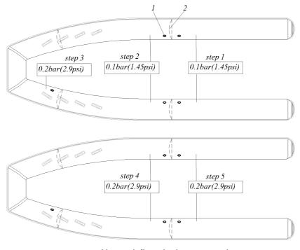
How to inflate the buoyancy tube. Fig.4a 1 - Inflation valve, 2 - partition
