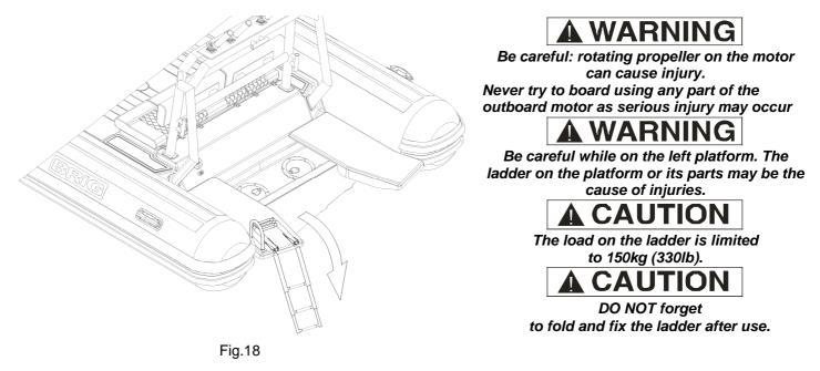
Be sure to use a hand hold for support as needed when on the ladder. Never try to board using any part of the outboard motor as serious injury may occur.
