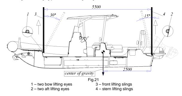
There are two bow eyes (1) and two aft eyes (2) installed to lift your boat. Always use all four eyes to lift the boat. You should always use only certified, verified and suitable lifting slings for lift of your boat.
