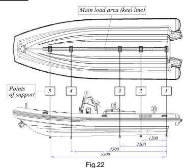
Installed on a trailer (or on kell-blocks for storage) the boat should been laying on all surface of the **Main loading area** (keel line) (Fig.22).
